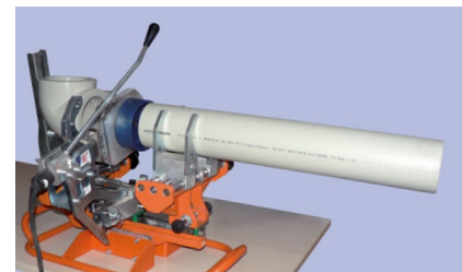
fixing and aligning the components, then heating them up
