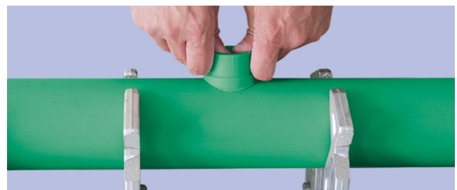
④ Install the heated up saddle in the heated hole and affix them there. After an hour, you can fill the system with water and expose it to the proper pressure.
