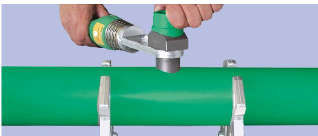
③ Mount the weld-in saddle on the heating extension piece and align the saddle and the extension piece guiding marks. Heat up the hole and the weld-in saddle.
